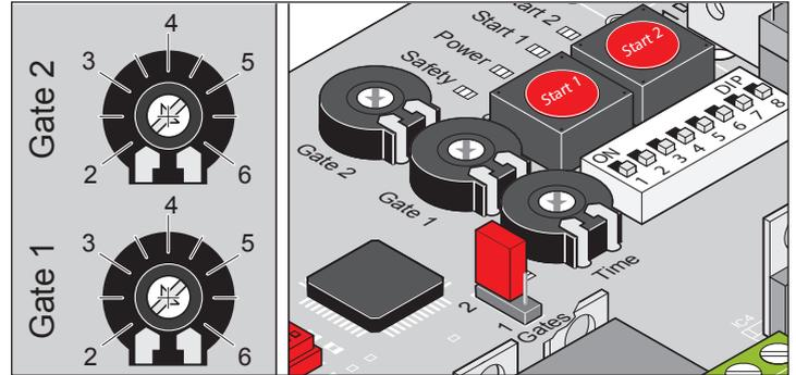
The length of the gate leaf is set at the control unit with the “Gate 1 (M1) + Gate 2 (M2)” potentiometers. The speed of movement and the force tolerance for the separate leaves of the gate installation are determined based on this setting.
