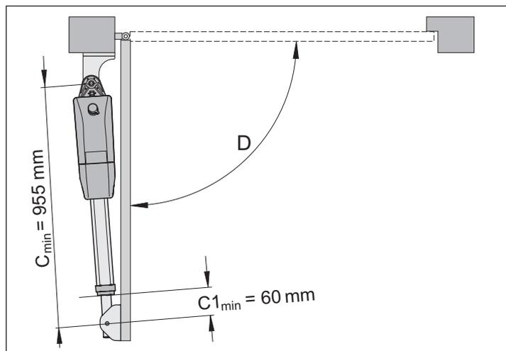
6. Manually move the gate to the "Gate OPEN" position. Note the maximum possible opening angle D from the A/B dimension table.
