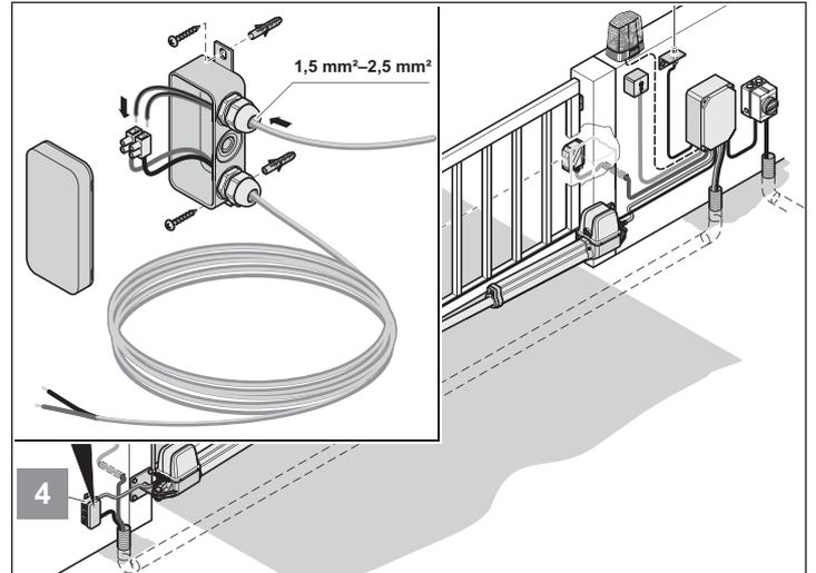
1. Fasten terminal box with screws through the eyelets.
