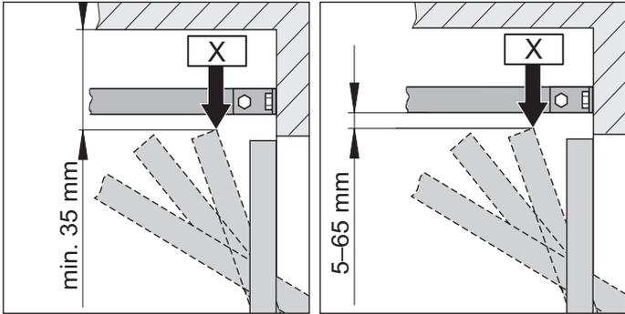
Fig. 1.1 Highest point for swing and up-and-over doors
