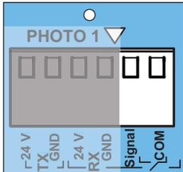
Fig. Terminal for 2-wire photo eye
