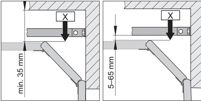
Fig. 1.2 Highest point for a sectional door
