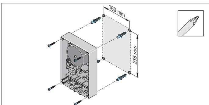
Fig. 3: Installation example
