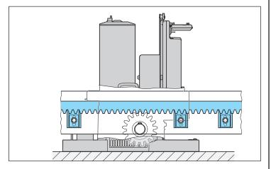
5. Remove the auxiliary mounting plates.
