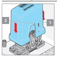
Remove the power supply cord provided and replace it with a permanently installed power supply cable.
