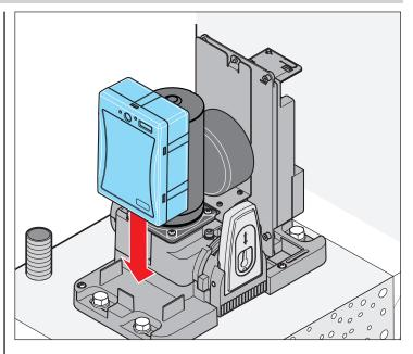
2. Position the battery pack in accordance with the illustration.
