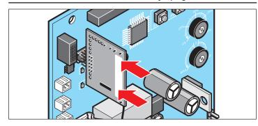
Connect the receiver pcb in accordance with the diagram on the control unit.
