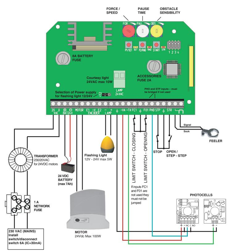
**NOTE:** The control unit is supplied with a trimmer to adjust the force of the motors set on maximum value (100%). Maintain this setting, which facilitates installation in difficult conditions (worn-out or not lubricated hinges, stress points etc.) Afterwards, reduce the force to obtain an operator movement that is slower and requires less force. After having adjusted the force the learning procedure must be repeated.
