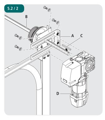
Fit the torque support bracket/console (A).
