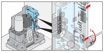
Left stop of potentiometer (–) is the lowest force tolerance, right stop (+) is the highest tolerance.
