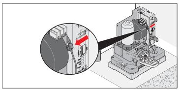
1. Connect the earth wire (factory-installed) to the earth clamp (see diagram).
