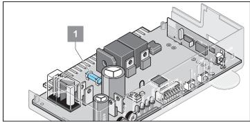
Open control unit housing and replace faulty fuse (1). Fuse "1A – fast-acting" for warning light-1 connection, terminal 16 + 17.
