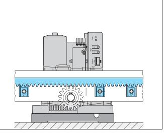
5. Remove the auxiliary mounting plates.
