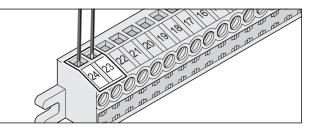
Terminals 23 + 24 Max. switching capacity: AC 230 V, max. 5 A The "max. switching duration" can only be changed with the TorMinal.
