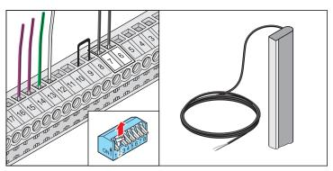
Terminal 6 + 7 DIP switch 2 Tested connection for an 8.2 kohm strip
