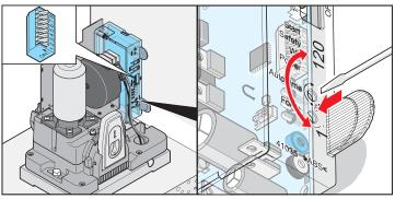
Switch open hold time on and off with potentiometer:
