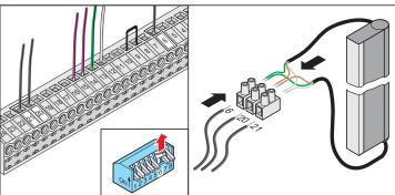
Terminal 6 Terminal 20 Terminal 21 DIP switch 6 DIP switch 2 Green cable from Fraba System Brown cable from Fraba system White cable from Fraba system ON OFF
