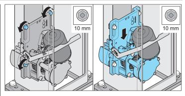
Tip! Mark the position of the motor unit before loosening the bolts.
