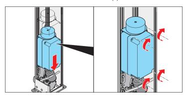
4. Lower the control unit approx. 150 mm and fix in place again.
