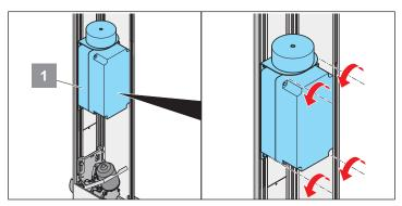
3. Unscrew the 4 screws on the control unit (1).
