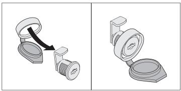
1. Assemble dust cap and lever lock as shown in the diagram.
