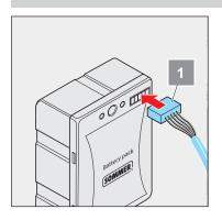
9. Plug connector cable into the battery pack (1).
