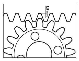
The play between pinion and racks must be approx. 1.5 mm.
