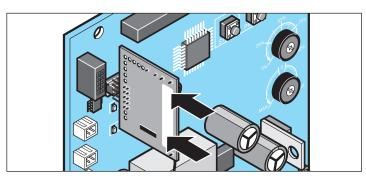
1. Connect the receiver board to the control unit as shown in the diagram.
