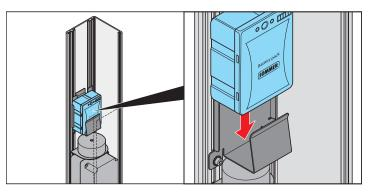
10. Place battery pack on the installation plate.
