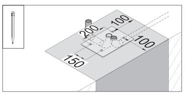
2. Measure and mark the drill holes for the foundation.
