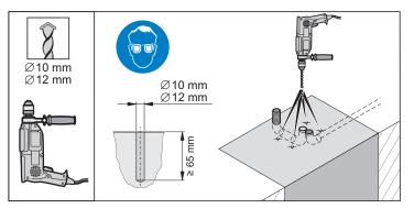
3. Drill four holes Ø 10 or Ø 12 mm and at least 65 mm deep.
