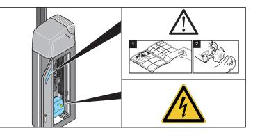
The following warning signs must be attached by the installer/operator:
