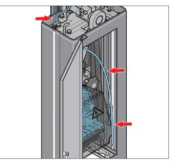
Route cables into the boom housing through the base plate cable gland.
