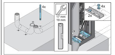
4. Blow out holes with compressed air.
