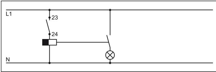
**Example: Staircase lighting with automatic switching system**
