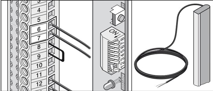
Terminal 6 + 7: Tested adapter for 8.2 kOhm resistor
