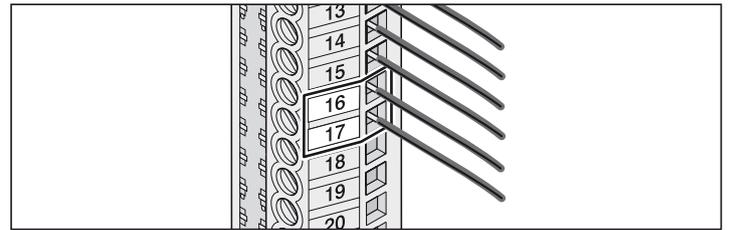
Terminal 16 + 17 unregulated DC 24 V (max. 34 V) 25 Watt, max. 1 A
