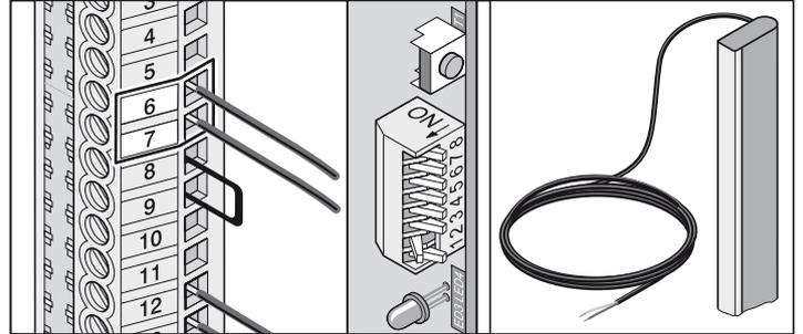
Terminal 6 + 7 Tested adapter for 8.2 kOhm resistor
