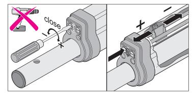
If necessary, readjust end position with a screwdriver.
