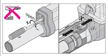
If necessary, readjust end position with a screwdriver.
