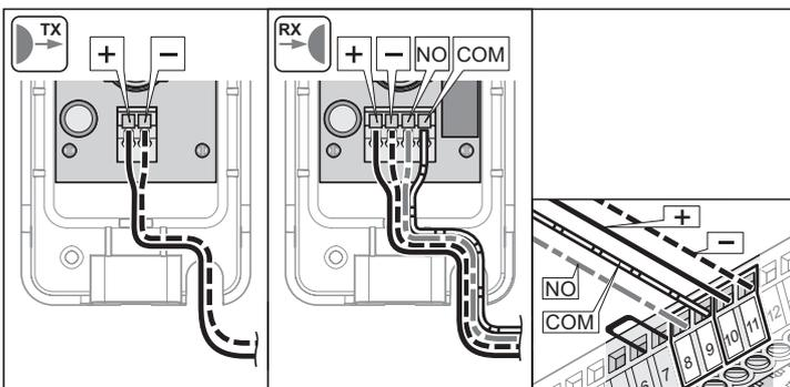
Terminals 8 + 9 Tested connection for floating contacts, **reacts only with door open.**
