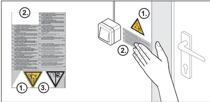
Please attach the warning signs (text + triangle sign) to a position where they are clearly visible, e.g. beside the pushbutton (warning triangle) and on the door wing (text + warning triangle).
