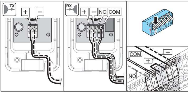
Terminals 6 + 7 Tested connection for floating contacts, **only if DIP switch 2 OFF.**
