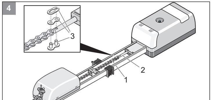
**4** The chain (1) is connected to the chain attachment bolt of the controller housing (2) by means of the chain lock (3).
