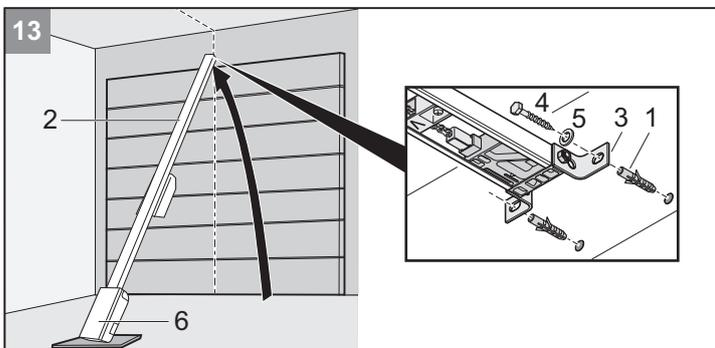
**13** Insert anchor fittings (1). Lift the drive (2) at the front. Tightly fasten header fitting (3) at the front with two bolts (4) and U-washers (5).
