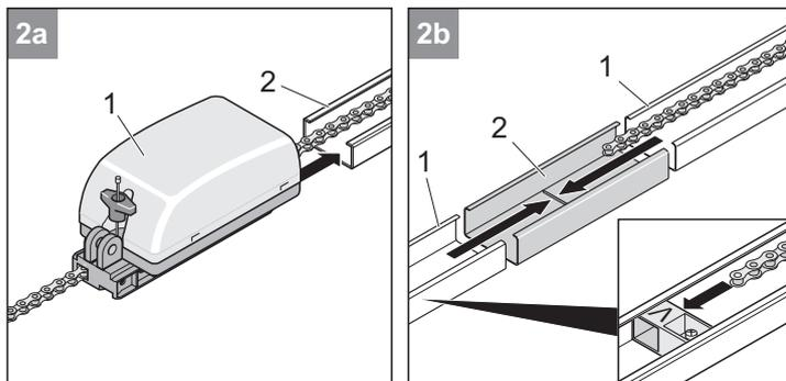
**2a** Put the carriage contact springs in place. Slide the carriage (1) with chain onto the rails (2) with the red guide idler "H". The tip of the guide idler must point toward the carriage (1). Push the chain through the red guide idler "H".
