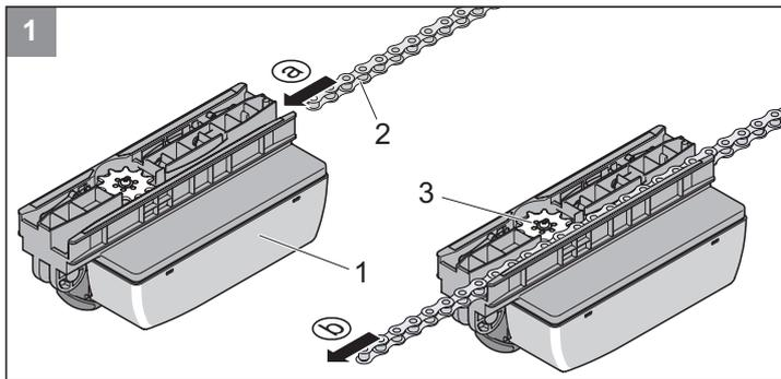
**1** Insert the chain (2) from behind into the carriage (1). Ensure that the chain (2) lies correctly on the chain wheel (3).
