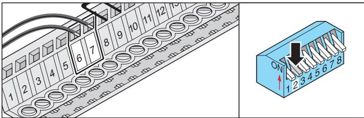
Terminals 6 + 7 Tested connection for an 8.2 kOhm resistor, **DIP switch 2 OFF.**
