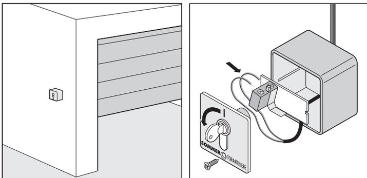
**19** Install the key switch (1) in a suitable, easily accessible position in the garage. Minimum height above the ground: 1.6 m.
