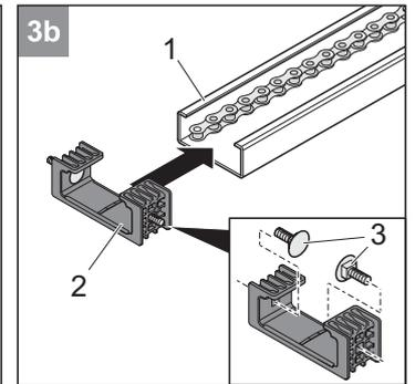
**3b** Push the controller housing up to the stop position at the rear of the rail and put the carriage contact springs in place. Make sure that the chain attachment bolt of the controller housing runs on the same side as the chain.
