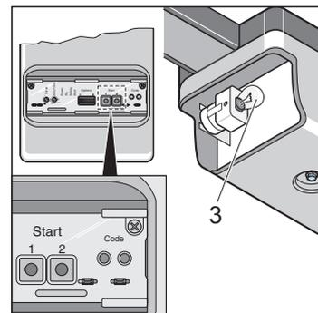
1. Press buttons 1 + 2 until the light bulb (3) extinguishes.
