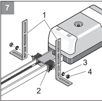
**7** Mount the two steel brackets (1) with washers (4) and toothed lock washers (3) onto the ceiling holder (2).
